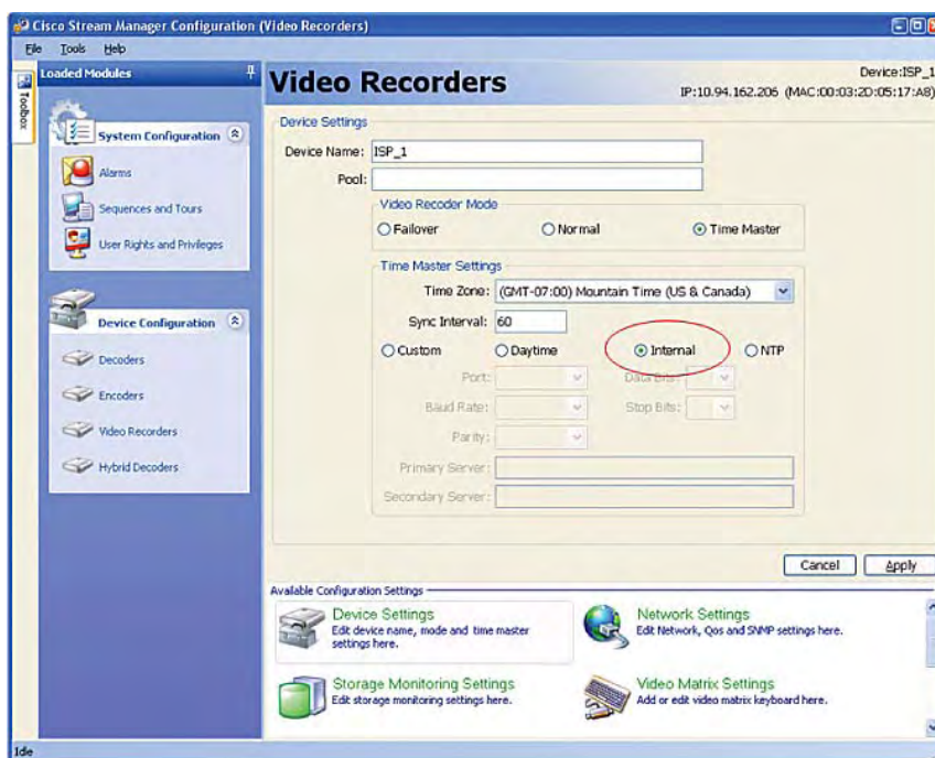
Figure 30. Time Synchronization with Internal clock
