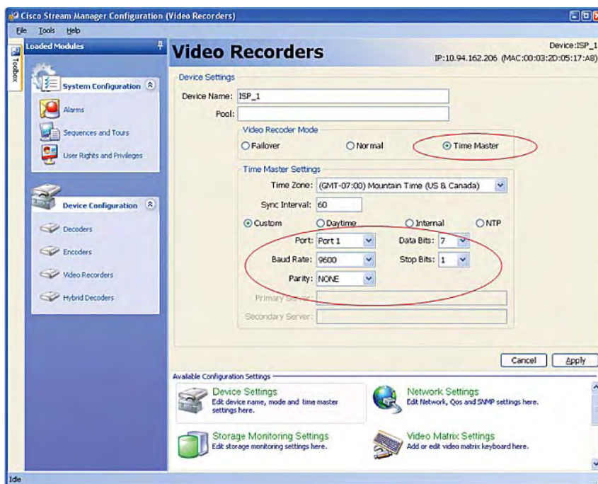
Figure 29. Time Synchronization from Matrix Switch
