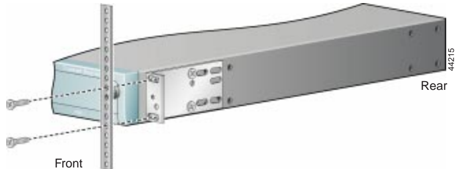
Figure 3-6 Installing the Chassis in the Rack
