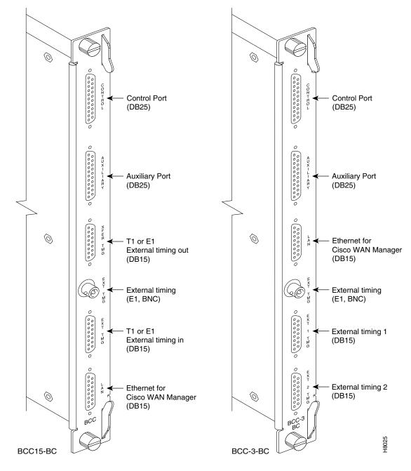
Figure 3-5 BCC-3-bc or BCC-c Face Plate Connectors
