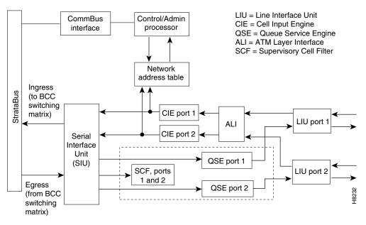
Figure 5-7 ASI-155 Simplified Block Diagram
