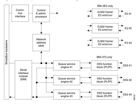
Figure 4-2 Simplified BNI-T3, BNI-E3 Block Diagram
