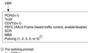
1 = VBR.1 2 = VBR.2 3 = VBR.3 4 = PCR policing only 5 = policing off Note: BW allocation = (PCR)x(%Util)
