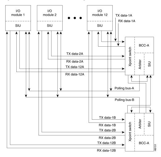
Figure 3-2 BCC-32 and BCC-3 Block Diagram
