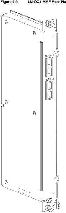
Figure 4-9 LM-OC3-MMF Face Plate
