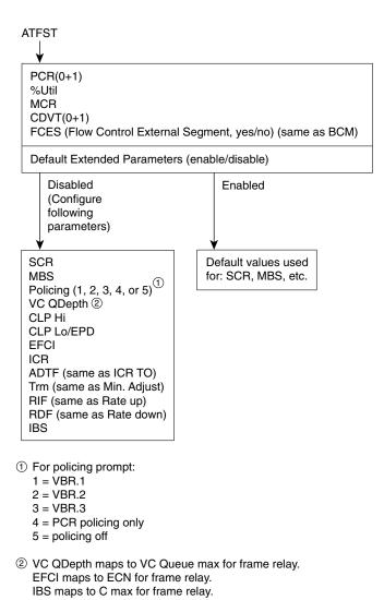
Note: FBTC (Frame based traffic control - AAL5, same as FGCRA) is automatically set to yes.
