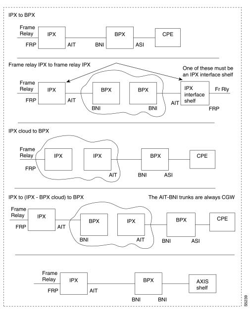
Figure 10-3 Frame Relay to ATM Interworking Examples with AIT Card on IPX
