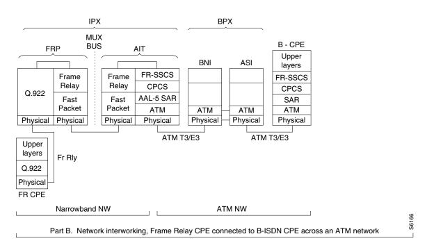
The Frame Relay to ATM networking interworking function is available as follows:
