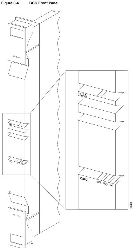
The BCC runs self-tests continuously on internal functions in the background and if a failure is detected, the **fail** LED is lighted. If the BCC is configured as a redundant pair, the off-line BCC is indicated by the lighted **stby** LED. The **stby** LED also flashes when a software download or standby update is in progress. The LAN LED indicates activity on the Ethernet port.
