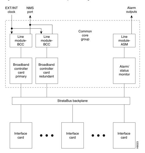
Figure 3-1 Common Core Group Block Diagram
