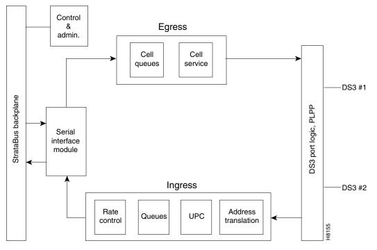
Each port provides an aggregate ATM connection bandwidth of 96,000 cells/second (T3) or 80,000 cells/sec (E3), or 353,208 cells/sec (OC3).
