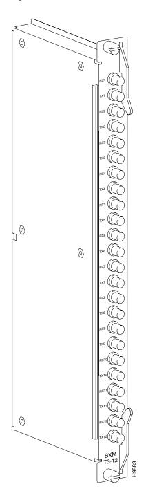
Figure 6-7 BPX-T3/E3 Back Card, 12-Port Option Shown
