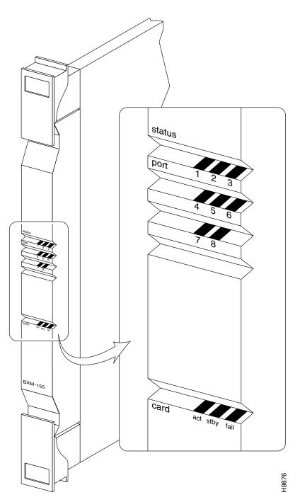
Figure 6-3 BXM-155 Front Panel, Eight-Port Card Shown
