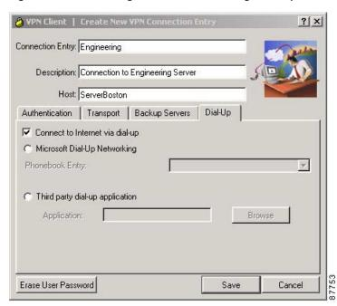
Figure 4-6 Connecting to the Internet Through Dial-up
