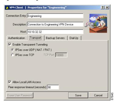
Figure 1-5 Setting the Allow Local LAN Access Parameter on the VPN Client
