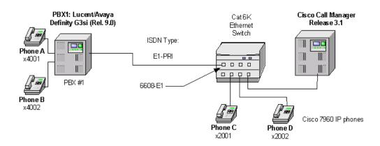
As shown in the figure above, a Lucent/Avaya Definity G3si PBX was connected via an ISDN E1 PRI link to a Cisco 6608-E1 Gateway, which in turn, was connected to an Ethernet switch. The interoperability testing involved Layers 1, 2 and 3 on the ISDN PRI link between a Cisco 6608-E1 and the PBX.
