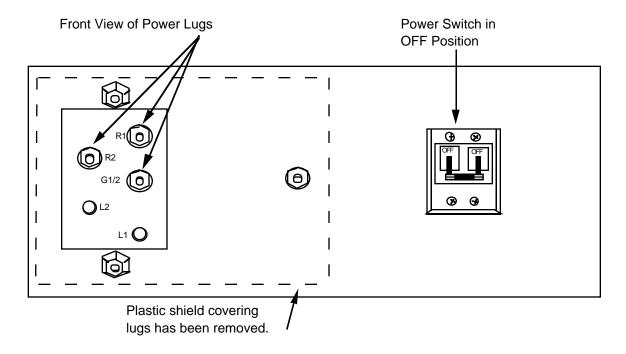
Figure 2: Front View of Power Distribution Box
