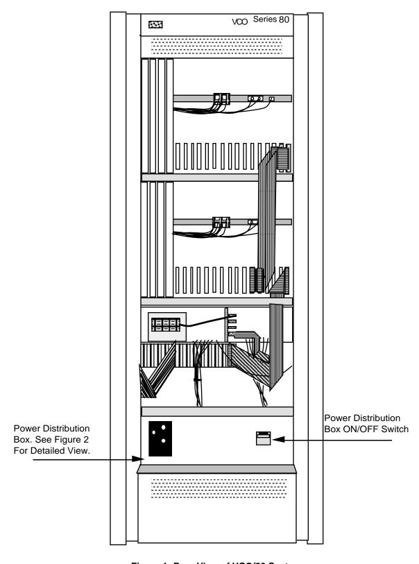
Figure 1: Rear View of VCO/80 System
