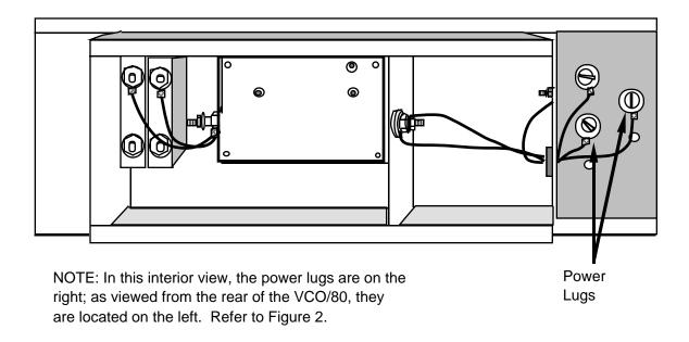
Figure 3: Interior View of Power Distribution Box
