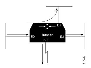
A directed broadcast address includes the network or subnet fields. For example, if the network address is 128.1.0.0, the address 128.1.255.255 indicates all hosts on network 128.1.0.0. This would be a directed broadcast. If network 128.1.0.0 has a subnet mask of 255.255.255.0 (the third octet is the subnet field), the address 128.1.5.255 specifies all hosts on subnet 5 of network 128.1.0.0— another directed broadcast.
