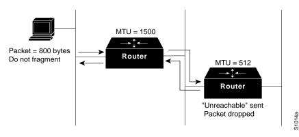
message to the source of the datagram with its Code field indicating "Fragmentation needed and DF set." To support Path MTU Discovery, it also would include the MTU of the next-hop network link in the low-order bits of an unused header field.
