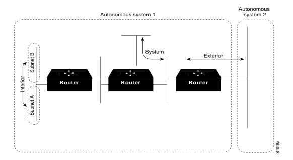
System routes are routes to networks within an autonomous system. The router derives system routes from directly connected network interfaces and system route information provided by other IGRPspeaking routers. System routes do not include subnet information.
