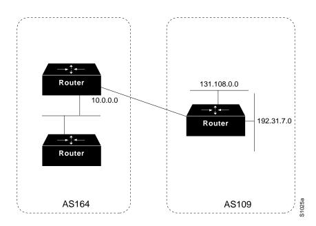
Figure 1-12 Router in AS 164 Peers with Router in AS 109
