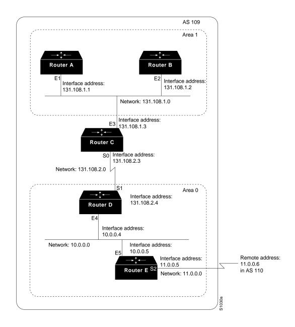
In this configuration, five routers are configured in OSPF autonomous system AS 109:
