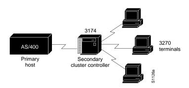
The 3270-style terminals attached to the 3174 controller cannot initiate a data transfer because the 3174 is the secondary node on the link. The primary host ensures a reasonable response time for its secondary nodes by sending out polls at a rate that is often more than 20 times per second. With two devices sharing a single, dedicated serial line, as in the preceding example, this poses no problem, because the link would be idle without the polls.
