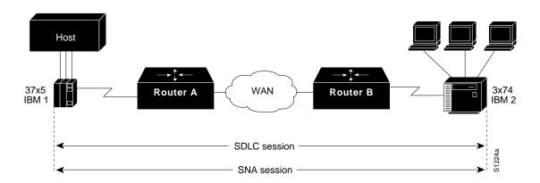
With SDLC Local Acknowledgment, the SDLC session between the two IBM end nodes is not endto-end but instead terminates at the two local routers, as shown in Figure 1-2. The SDLC session with IBM 1 ends at Router A, and the SDLC session with IBM 2 ends at Router B. Both Router A and Router B execute the full SDLC protocol as part of SDLC Local Acknowledgment. Router A
