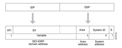
The ISO-IGRP NSAP address is divided into three parts: a domain part, an area address, and a system ID. Domain routing is performed on the domain part of the address. Area routing for a given domain uses the area address. System ID routing for a given area uses the system ID part. The NSAP address is laid out as follows:
