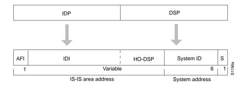
The IS-IS routing protocol interprets the bytes from the AFI up to (but not including) the system ID field in the DSP as an *area identifier*. The system ID specifies the *system*.
