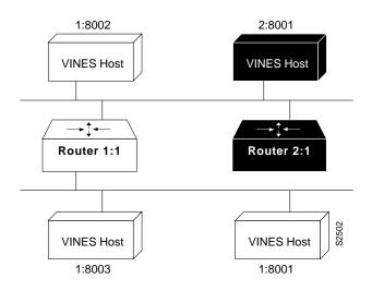
The subnetwork number is 16 bits (2 bytes) long. For service nodes, this the subnetwork number is always 1. For client nodes, it can have a value from 0x8001 through 0xFFFE.
