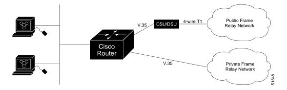
The frame relay interface actually consists of one physical connection between the network server and the switch that provides the service. This single physical connection provides direct connectivity to each device on a network, such as a Stratacom FastPacket wide-area network, using only a single connection.
