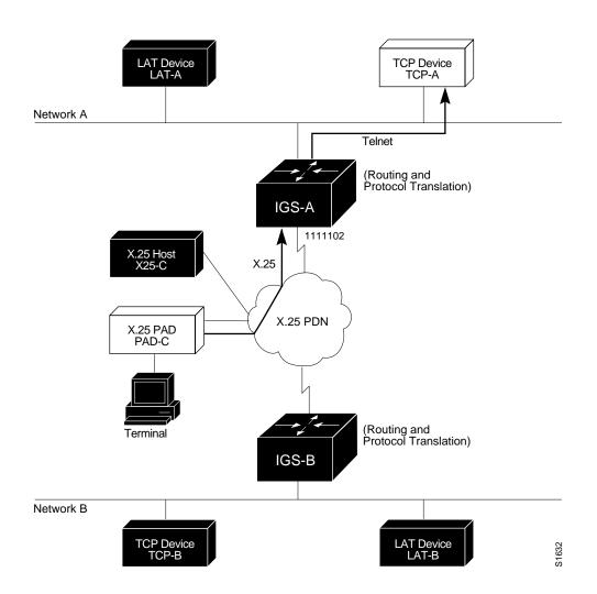
The following example configuration illustrates use of the **translate** global configuration subcommand to translate from an X.25 PAD to a TCP-device on Network A. It is applied to IGS-A.
