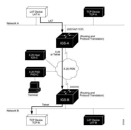
The following configuration examples illustrate use of the **translate** global configuration subcommand to translate from LAT to X.25 (IGS-A) and from X.25 to Telnet (IGS-B) allowing connection service to a TCP-device on Network B (TCP-B) from a LAT-device on Network A (LAT-A). Example configurations are for both IGS-A and IGS-B.
