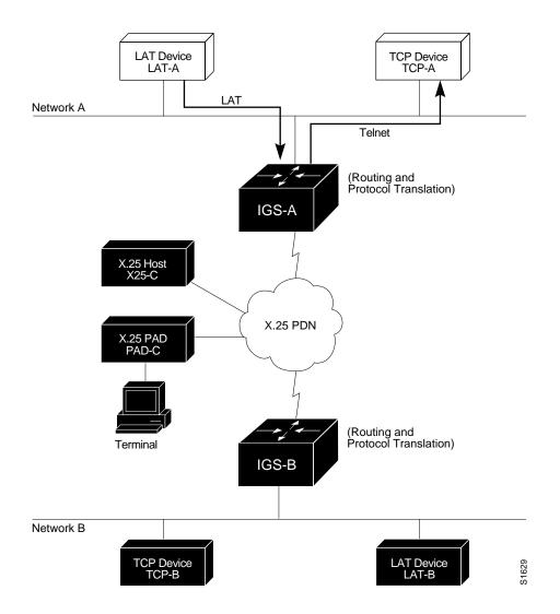
The following example configuration illustrates use of the **translate** global configuration subcommand to translate from LAT to TCP. It is applied to IGS-A.
