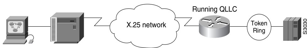
Figure 166 Router Running QLLC Conversion Feature
