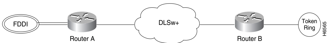
Figure 136 DLSw+ Translation Between FDDI and Token Ring
