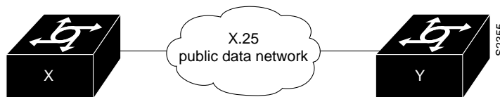
Figure 8-1 Transporting LAN Protocols across an X.25 PDN
