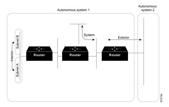
System routes are routes to networks within an autonomous system. The router derives system routes from directly connected network interfaces and system route information provided by other IGRPspeaking routers. System routes do not include subnet information.
