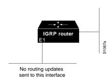
As in the first example, IGRP updates are sent to all interfaces on network 131.108.0.0 except interface Ethernet 1 in the following example. However, in this case a **neighbor** router configuration command is included. This command permits the sending of routing updates to specific neighbors. One copy of the routing update is generated per neighbor.
