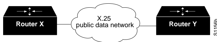
Figure 11-1 Transporting LAN Protocols across an X.25 PDN
