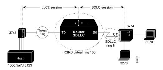
The following sample configuration file is for SDLLC with a single router using RSRB:
