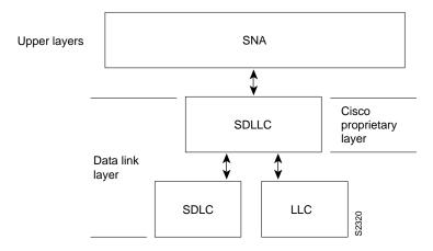
As Figure 1-1 shows, SNA uses SDLC and LLC2 as link-layer protocols to provide a reliable connection. The translation function between these industry-standard protocols takes place in the proprietary Cisco software.
