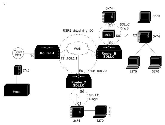
The following configuration files describe the network shown in Figure 1-6. The note references to the right of the configuration files refer to the "Notes" section at the end of this chapter.
