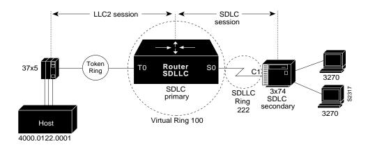
Figure 1-3 SDLLC Communication between a 37x5 and a 3x74 Connected to the Same Router (Direct Connection)
