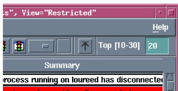
Figure 13: Restricting Rows Displayed in the Event List - the Top [Min-Max] Text Box
