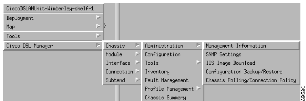
Figure C-1 Cisco DSL Manager Menu—Chassis Administration
