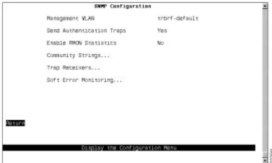
Figure 6-15 SNMP Configuration Panel
