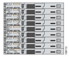
In this example, the stacks use both the 0.5- and the 3-meter StackWise cables to make redundant connections.
