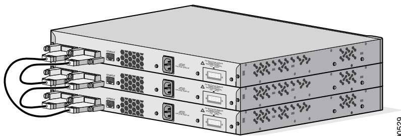
Figure C-2 Stacking the Switches
