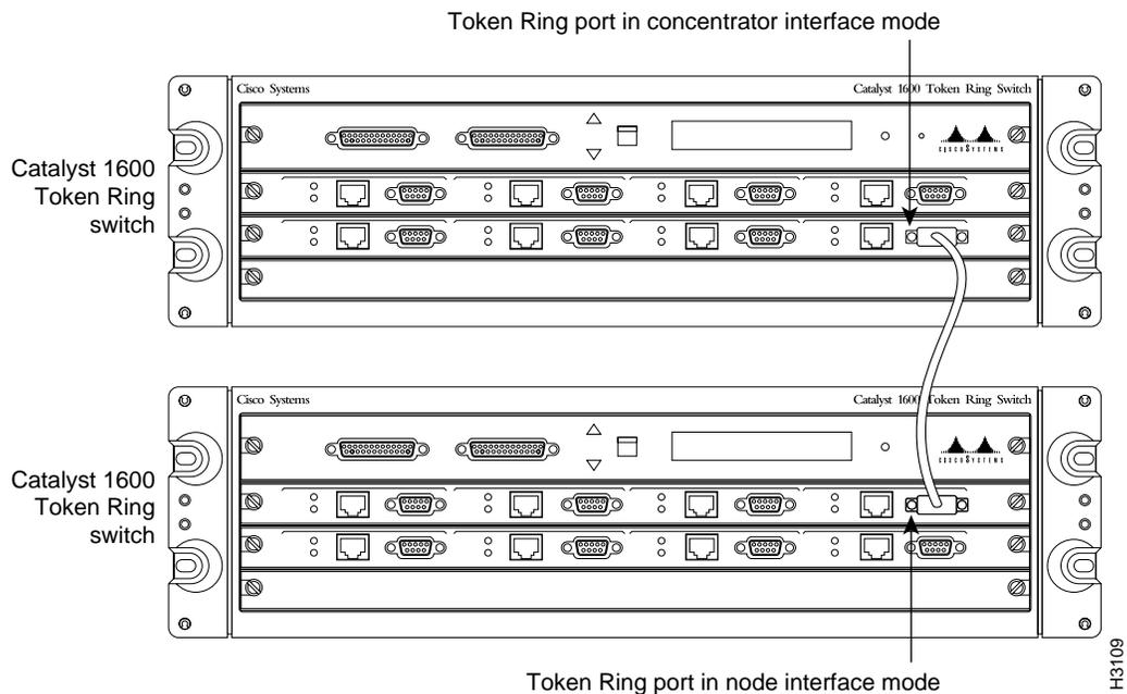
When you connect two Catalyst 1600 devices by their Token Ring ports, make sure the ring number is identical for both Token Ring ports.
