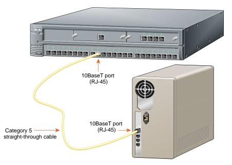
Note: Use a straight-through cable to connect two ports when one of the port numbers is designated with an X. Use a crossover cable to connect two ports when both port numbers are designated with an X. These cables are not supplied with the switch.
