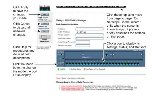
You can use the Switch Manager to change the switch configuration and to monitor switch conditions and statistics from anywhere on your intranet.
