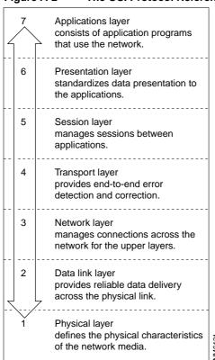
Figure A-2 The OSI Protocol Reference Model
