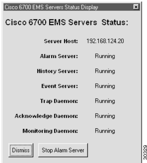
Figure 12-2 Alarm Server Status Window
