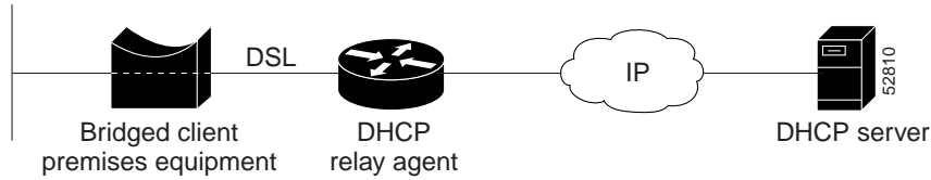
Figure 6-1 Network Topology Using ATM RBE and DHCP
