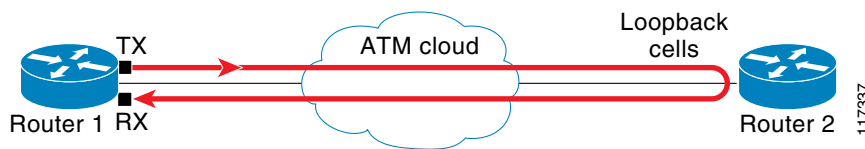
Figure 8-3 Performing a Local Loopback—Router Level
