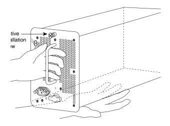
This procedure applies to AC-input and DC-input power supplies, with differences clearly noted. Do not mix AC-input and DC-input power supplies in the same chassis. Install the first power supply in the lower power supply bay and the second, if any, in the upper bay. In systems with dual power supplies and
