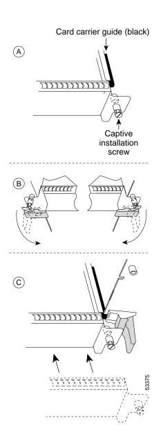
The Route Switch Processor (RSP) comes uninstalled with your Cisco 7507 router, but is a required system component. Install the RSPs in the slot 2 or slot 3, and install any interface processors, fillers, or Versatile Interface Processors (VIPs) in slots 0, 1, 4, 5, and 6 (optional).
