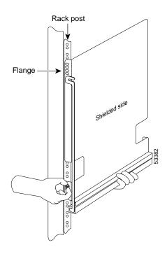
**Note** The distance between the inner edges of the left and right rack-mounting posts must be at least 17.72 inches (45.088 cm), and the distance between the holes in the mounting posts must be 18.31 inches (46.5 cm) ( $\pm$  .063 inches or .16 cm).
