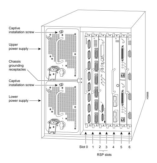
The Cisco 7507 has seven slots: slots 2 and 3 for the Route Switch Processors (RSPs), and slots 0, 1, 4, 5, and 6 for the interface processors. There are bays for up to two AC-input or DC-input power supplies. One power supply is shipped as standard equipment; a second power supply is optional. A second (optional) power supply allows load sharing and increased system availability.
