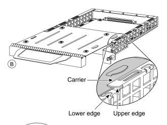
**Note** First remove the VIP from the chassis before removing the port adapter from the VIP. See the "Remove and Install an Interface Processor, Filler, VIP, or RSP" section on page 29 for instructions.
