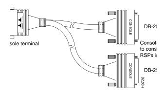
The console and auxiliary Y-cables allow you to simultaneously connect the console or auxiliary ports on two RSP2s, RSP4s, or RSP8s, to a single console terminal, or external auxiliary device. These are configured as system master and slave in slots 2 and 3 in the Cisco 7507.
