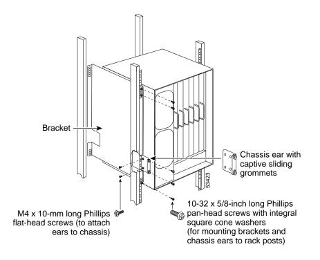
To rack-mount a Cisco 7507 router, perform the following steps:
