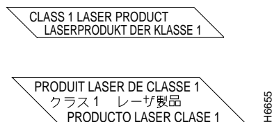
Figure 6 Laser Warning Labels on POSIP for Single Mode
