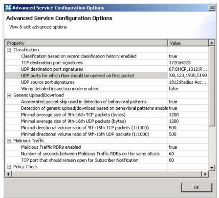
Step 2. In the Advanced Service Configurations Options dialog box, add port 5190 to the list of "UDP ports for which flows should be opened on first packet."
