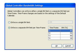
The "BW (%)" cell of the Global Controller Settings dialog box displays four different BW limits, one for each time frame, as illustrated in the following figure.
