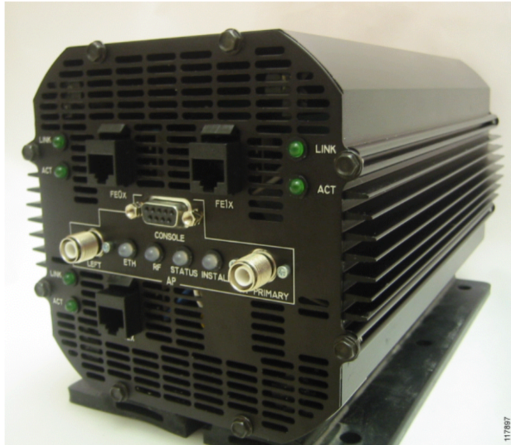
Figure 2-33 Example of a Configured Cisco 3200 Mobile Access Router with one MARC, Three FESMIC Ports, and One WMIC Port
