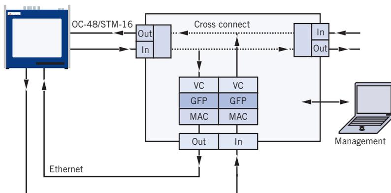
figure 6 Interworking test using the Acterna ONT-50
