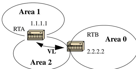
In this example, area 1 does not have a direct physical connection into area 0. A virtual link has to be configured between RTA and RTB. Area 2 is to be used as a transit area and RTB is the entry point into area 0. This way RTA and area 1 will have a logical connection to the backbone. In order to configure a virtual link, use the following router OSPF sub-command on both RTA and RTB:
