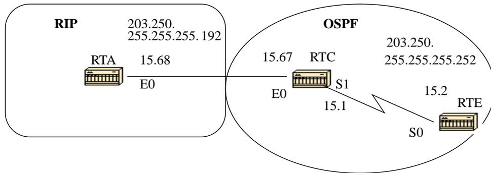
In the above diagram, RTE is running OSPF and RTA is running RIP. RTC is doing the redistribution between the two protocols. The problem is that the class C network 203.250.15.0 is variably subnetted, it has two different masks 255.255.255.252 and 255.255.255.192. Let us look at the configuration and the routing tables of RTE and RTA:
