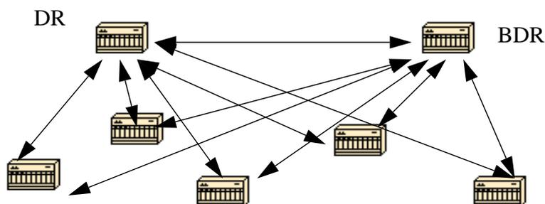
In the above diagram, all routers share a common multi-access segment. Due to the exchange of Hello packets, one router is elected DR and
