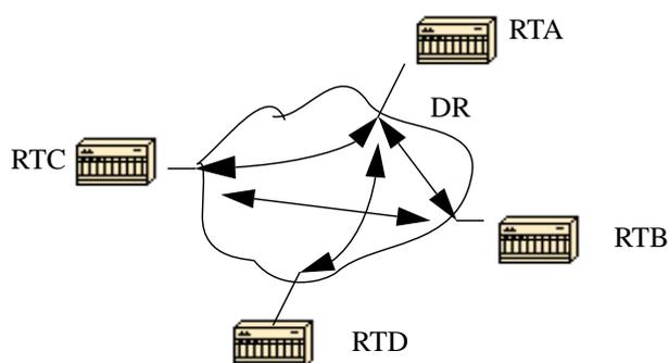
In the above diagram, it is essential for RTA's interface to the cloud to be elected DR. This is because RTA is the only router that has full connectivity to other routers. The election of the DR could be influenced by setting the ospf priority on the interfaces. Routers that do not need to become DRs or BDRs will have a priority of 0 other routers could have a lower priority.
