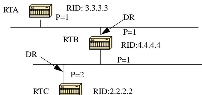
In the above diagram, RTA and RTB have the same interface priority but RTB has a higher RID. RTB would be DR on that segment. RTC has a higher priority than RTB. RTC is DR on that segment.
