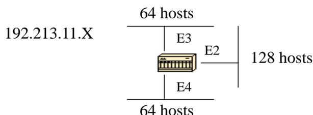
There are a handful of subnet masks that can be used; remember that a mask should have a contiguous number of ones starting from the left and the rest of the bits being all 0s.
