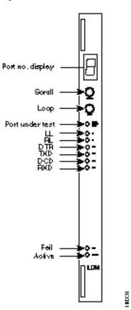
Figure 4-56 LDM Connections and Indicators
