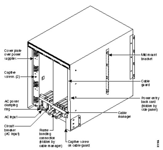
Figure 2-13 Power Supply Area Back View, AC System
