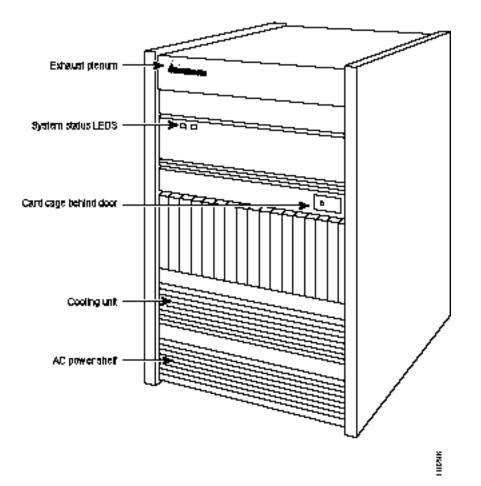
Figure 2-4 Component Locations IGX 8420 Standalone Switch
