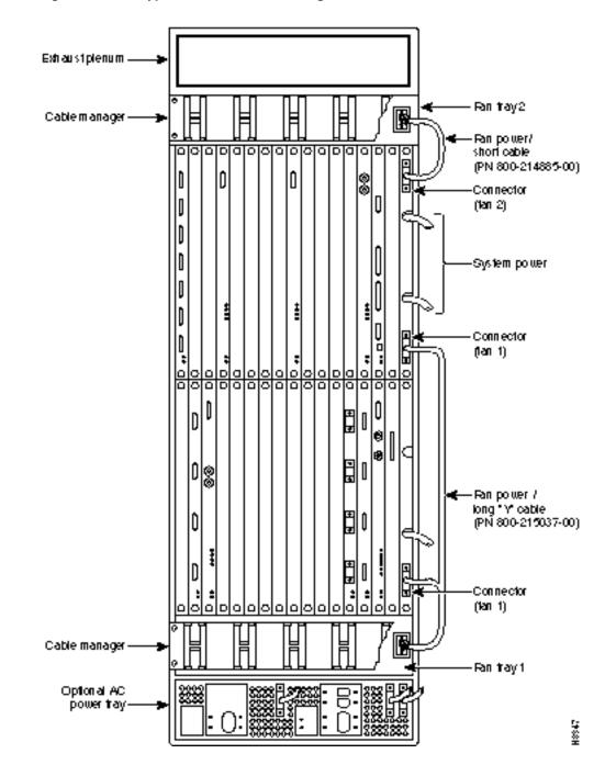
Figure 2-23 Typical IGX 8430 Shelf Configuration, Back View
