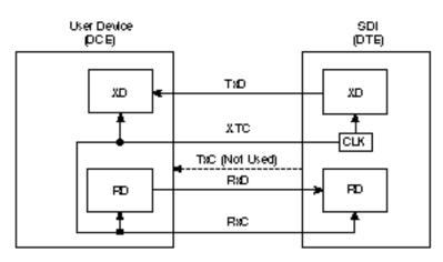
B. Loop Clock - User Device Loops Clock
