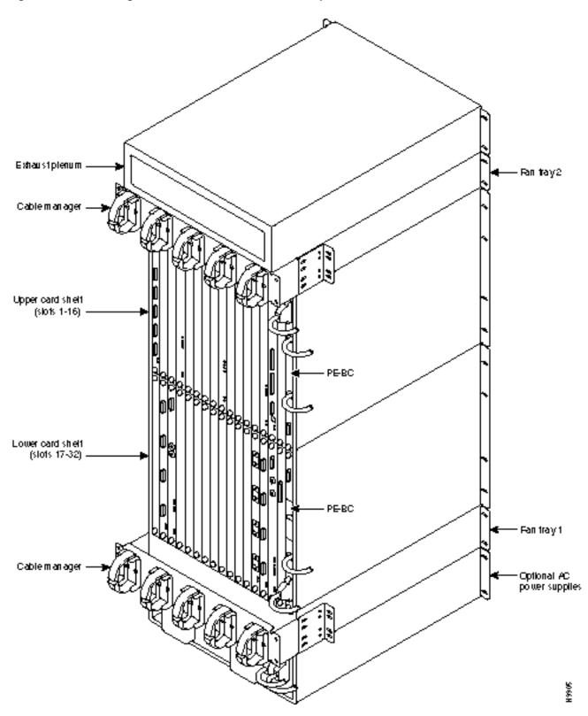
Figure 2-9 Stacking Order for IGX 8430 Rack-Mount Components, Back
