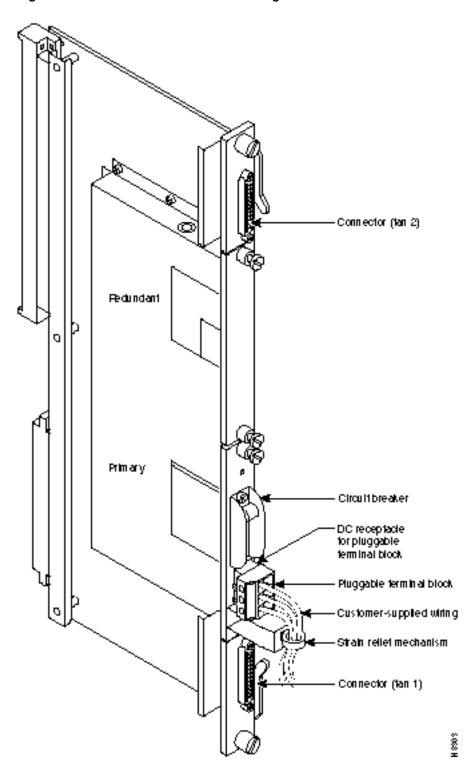
Figure 2-12 PE-BC and DC PEM With Plug
