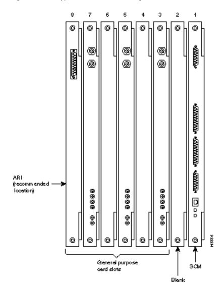
Figure 2-21 Typical IGX 8410 Shelf Configuration, Back View
