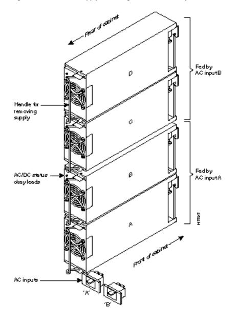
Figure 2-14 Power Supply Slot Designations, Dual AC System
