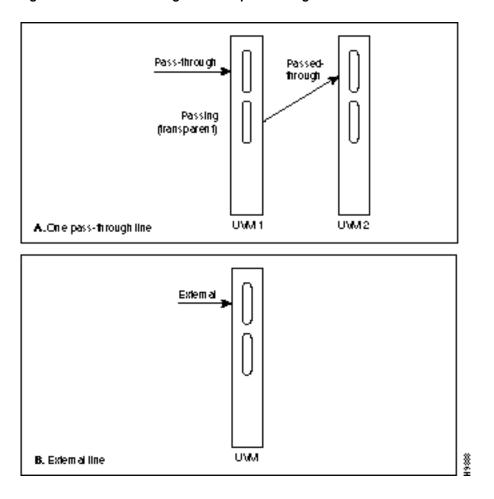
Figure 4-22 Pass-through and non pass-through modes for E1 or J1
