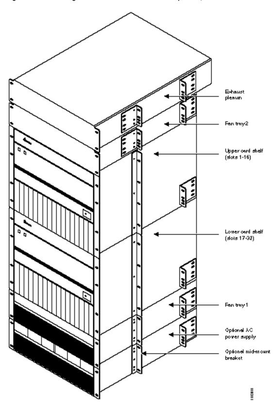
Figure 2-8 Stacking Order for IGX 8430 Rack-Mount Components, Front
