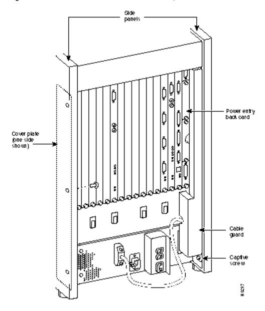
Figure 2-5 AC-Powered IGX 8420 Standalone Switch, Back View
