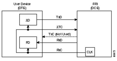
B. Loop Clock - User Device Loops Clock Leads
