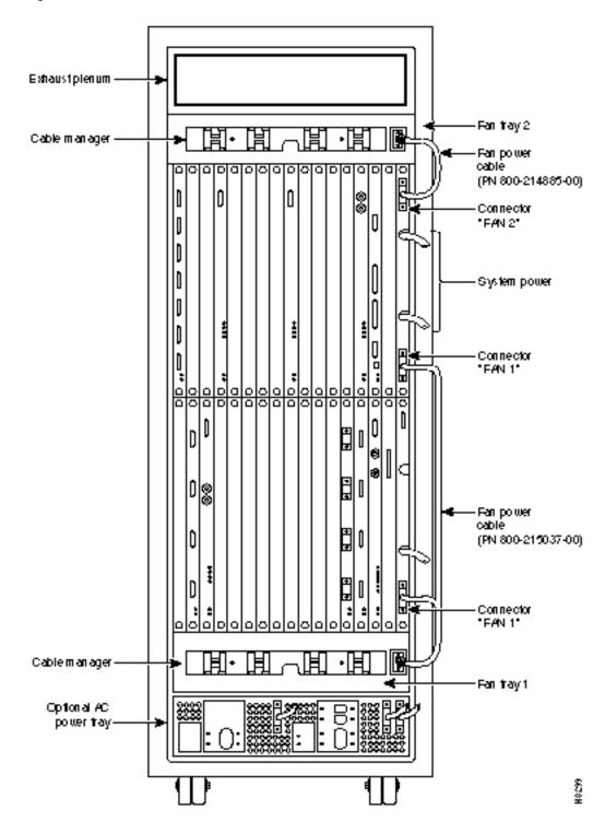
Figure 2-7 IGX 8430 Standalone Switch, Back View
