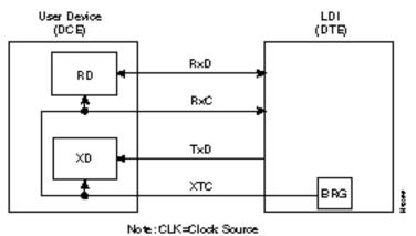
B.Looped Clock (LDI as a DTE) User Device Loops Clock
