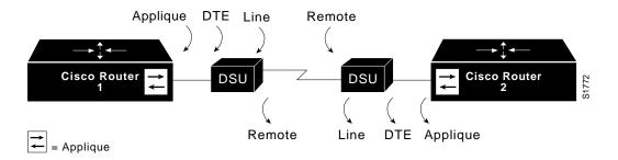
The subcommands to enable these tests are described next. In the following subcommands, the **loopback** command with no argument defaults to the **loopback applique** command.
