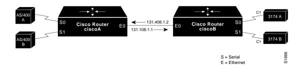
In the following configuration, the AS/400 device labeled A wants to communicate with the 3174 device labeled A, as do the AS/400 device labeled B and 3174 device labeled B. Notice that both of the 3174 devices are at SDLC address C1. A first attempt at the configuration files for the routers labeled ciscoA and ciscoB could be as follows.
