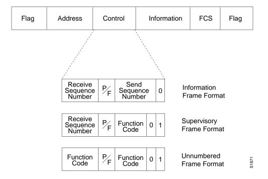
The Address field contains the address of a sending or receiving station, depending upon the procedure. The Control field contains information that determines the type of SDLC frame being transmitted, either:
