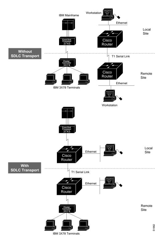
The software encapsulates SDLC frame traffic into IP packets and routes them over any of the IP-supported network media—serial, FDDI, Ethernet, and Token Ring, X.25, SMDS, and T1/T3—using the TCP transport mechanism. Because the TCP transport mechanism is used, you may use the Cisco IGRP routing protocol to route the packets. Use of IGRP allows load sharing of SDLC data for faster throughput.
