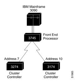
The configuration has a 3090 mainframe channel-attached to a 3745 controller, and these are connected by SDLC link to 3274 and 3174 cluster controllers.
