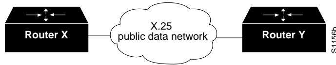
Figure 11-1 Transporting LAN Protocols across an X.25 PDN
