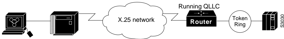
Figure 25-5 Router Running QLLC Conversion Feature
