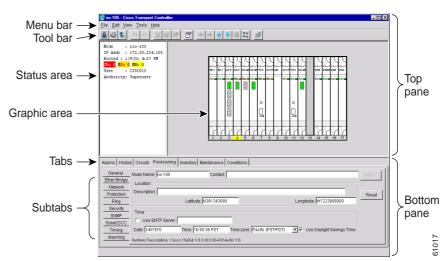
Figure 9 CTC GUI (window) in node view
