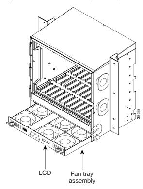
Figure 33 ONS 15454 fan-fray assembly
