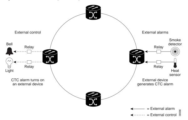
Provisioning external alarms and controls provides a "virtual wires" option that you can use to route alarms and controls from different nodes to one or more alarm collection centers. For example, in Figure 18, smoke detectors are provisioned as external alarms at Nodes 1, 2, 3, and 4. The alarms are assigned to Virtual Wire 1, and Virtual Wire 1 is provisioned as the trigger (control) for an external bell at Node 1.
