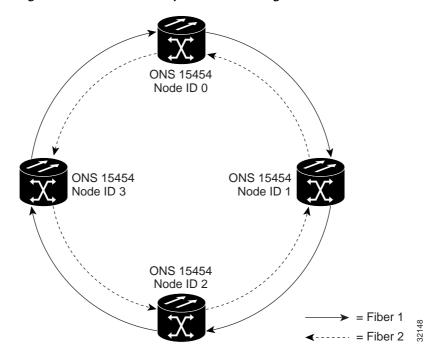
Figure 22 Unidirectional path switched ring
