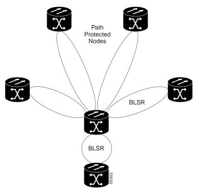
Figure 25 shows a UPSR subtending from a BLSR. In this example, Node 3 is the only node serving both the BLSR and UPSR. Optical cards in Slots 5 and 12 serve the BLSR, and optical cards in Slots 6 and 13 serve the UPSR.
