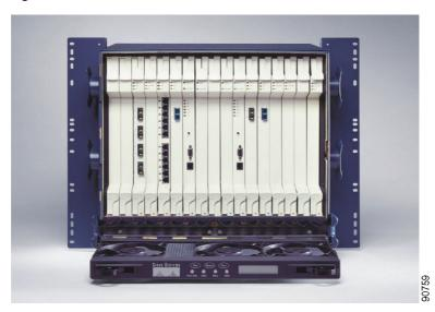
The ONS 15454 is a NEBS-compliant shelf assembly that contains 17 card (module) slots, a backplane interface, a fan tray, a front panel with an LCD, and alarm indicators. The ONS 15454 carries traditional time-division multiplexing (TDM) and high-speed data traffic—a variety of card configurations offer incremental bandwidth increases as needed and support EC-1, DS-1, DS-3, OC-3, OC-12, OC-48, OC-192, and 10/100/1000 Ethernet and Gigabit Ethernet speeds.
