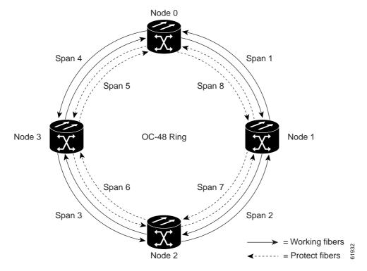
Four-fiber BLSRs double the bandwidth of two-fiber BLSRs by dedicating a second optical card for protection rather than reserving half of the active card for protection. If one fiber is cut, the ring does not switch because the other fiber carries the traffic for the broken span. A ring switch occurs if both the working and protect fibers fail. You can create OC-48 and OC-192 four-fiber BLSR.
