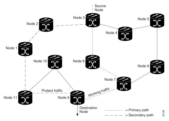
If you check the protected circuit box in CTC, PPMN establishes a second unique route between Nodes 3 and 9 and automatically creates cross-connections at nodes 3, 2, 1, 11, and 9, shown by the dashed line. If a signal failure occurs on the primary path, traffic switches to the second, protected circuit path. In this example, Node 9 switches from the traffic coming in from Node 7 to the traffic coming in from Node 11 and service resumes. The switch occurs within 50 milliseconds.
