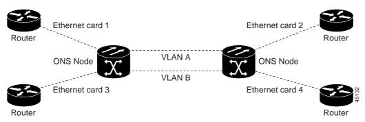
When you provision multicard EtherSwitch, two or more Ethernet cards act as a single layer 2 switch. Multicard EtherSwitch supports one STS-6c shared packet ring, two STS-3c shared packet rings, or six STS-1 shared packet rings. The bandwidth of the single switch formed by the Ethernet cards matches the bandwidth of the provisioned Ethernet circuit up to STS-6c worth of bandwidth.
