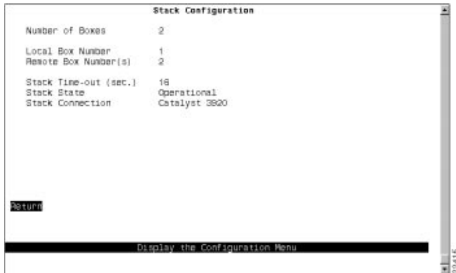
Figure 5-3 Stack Configuration Panel
