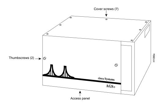
Figure 2 The Front and Top Panels on the A-Type Chassis
