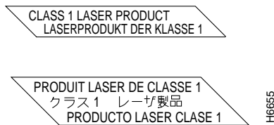
Figure 4-1 Laser Warning Labels for Single-Mode Port
