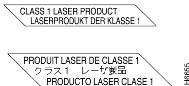
Figure 3-1 Class 1 Laser Warning Labels for Single-Mode Port
