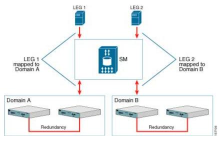
Figure 4-1: Cable Topology with Automatic Integration with a DHCP Server, Push Mode, and Fail-Over of SCE Platforms
