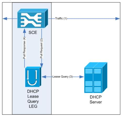
The subscriber's traffic (1) triggers a pull-request from the SCE (2). The Lease Query LEG receives the request and queries the DHCP server. If the server finds a match for the IP address in its database, the server replies with the subscriber information (3). Based on the received information, the LEG responds to the SCE with a pull-response, which includes the subscriber ID and the IP address lease-time returned from the DHCP server (4).
