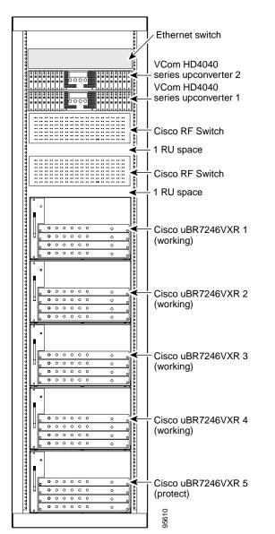
These illustrations show sample configurations using the Cisco uBR 3x10 RF Switch, upconverters, and the Cisco uBR7246VXR CMTS.
