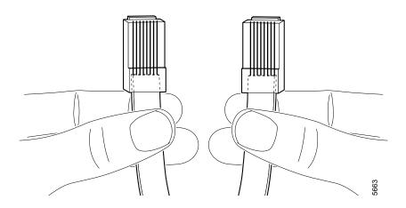
On a straight-through cable, the colored wires are in the same sequence at both ends of the cable.
